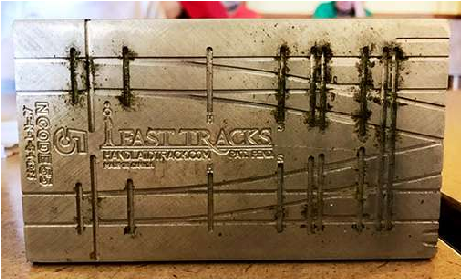
This is one of the jigs for a #5 turnout, right & left
