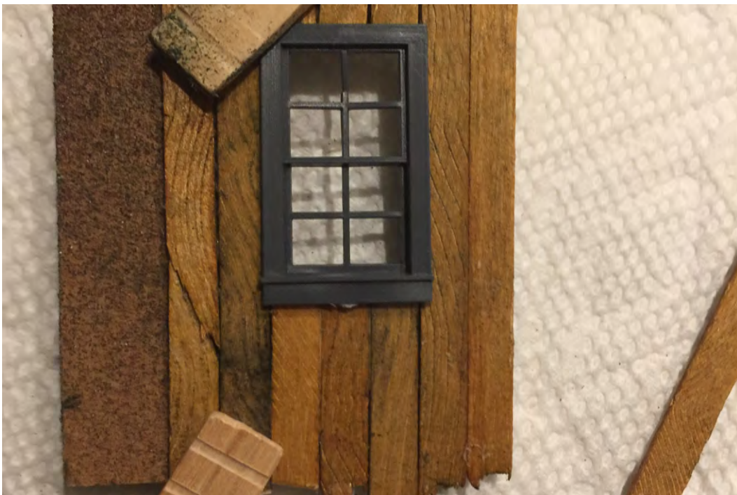
BEGINNING TO APPLY SIDE BOARDS TO PLYWOOD SUB-BASE (NOTICE THE PLYWOOD ON THE EXTREME LEFT) (PREVIOUSLY SEEN WHEN BEING CUT ON THE BANDSAW) (ALSO PLEASE NOTE THE GRANDT-LINE WINDOW... IT IS MERELY LAYING THERE NOT ADHERED, BUT USED FOR SPACING OF PLANKS AROUND THE OPENING)
