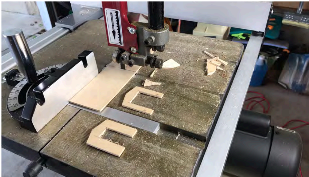
CUTTING PLYWOOD FOR "BACKING" SUPPORT OF THE ACTUAL CABOOSE, USING MY BANDSAW
