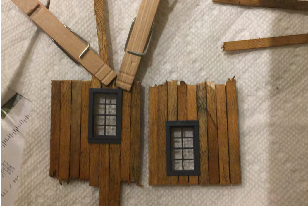
SIDE PLANKING APPLIED TO BOTH SIDES OF THE CABOOSE STRUCTURE
