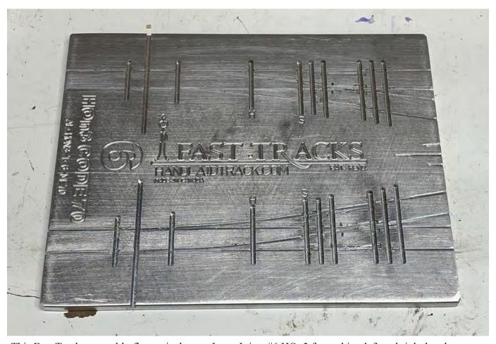
This Fast Tracks assembly fixture is the one I use. It is a #6 HOn3 for making left and right hand switches. I suspect you can imagine how quickly it can take the heat out of the rail you are trying to solder. Practice has helped, but it's still a little tricky for me.
