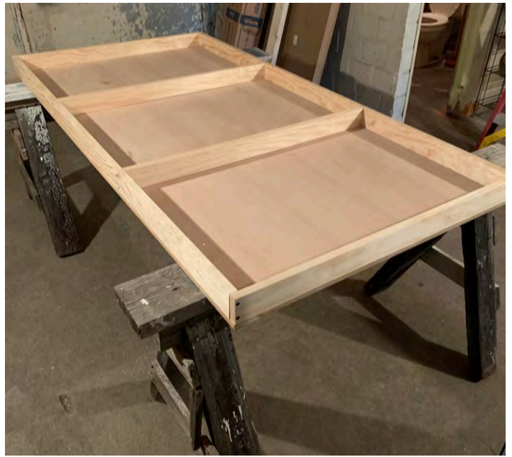
The pallet is made of 1/2" cabinet grade plywood with 1"x 3" support frame. I painted both the top and the underside with Kilz white primer to seal the wood.
