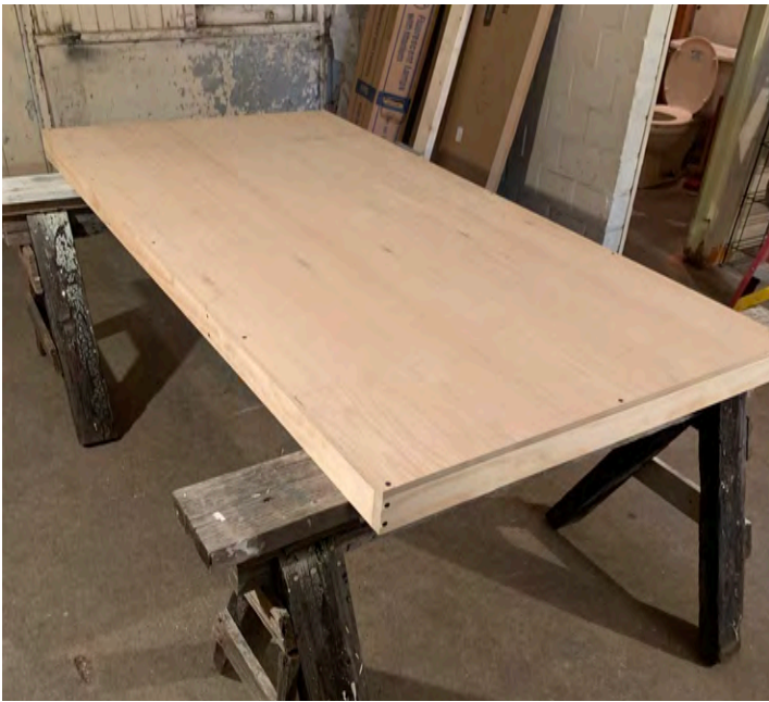
The pallet is made of 1/2" cabinet grade plywood with 1"x 3" support frame. I painted both the top and the underside with Kilz white primer to seal the wood.
