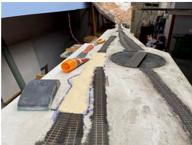
I patched the surface with Elmer's Wood Filler for indoor use, then sanded it flat. I find that I can spike through it as easily as I can the Homasote.
