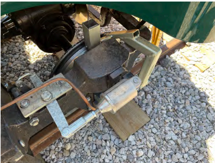
15) This is the front truck's flange lubricator and a brake cylinder.
