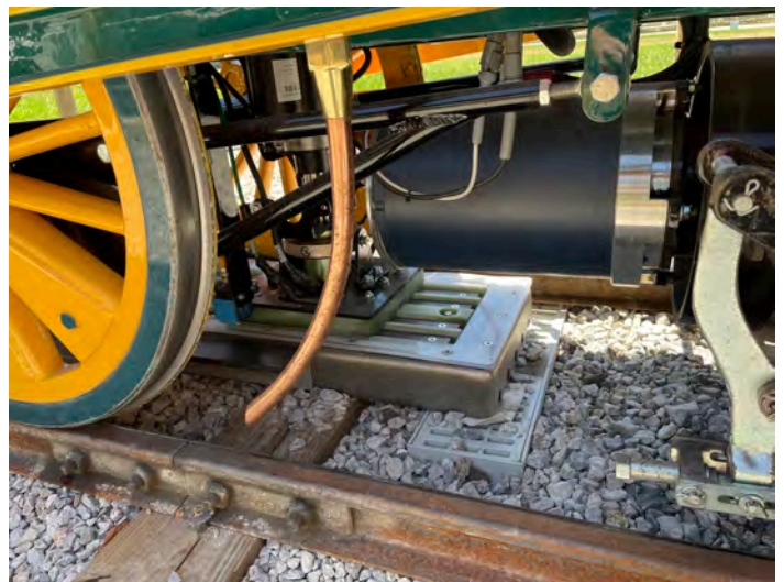
14) The charging shoe drops down on the plate to activate it. The black cylinder is the front motor.
