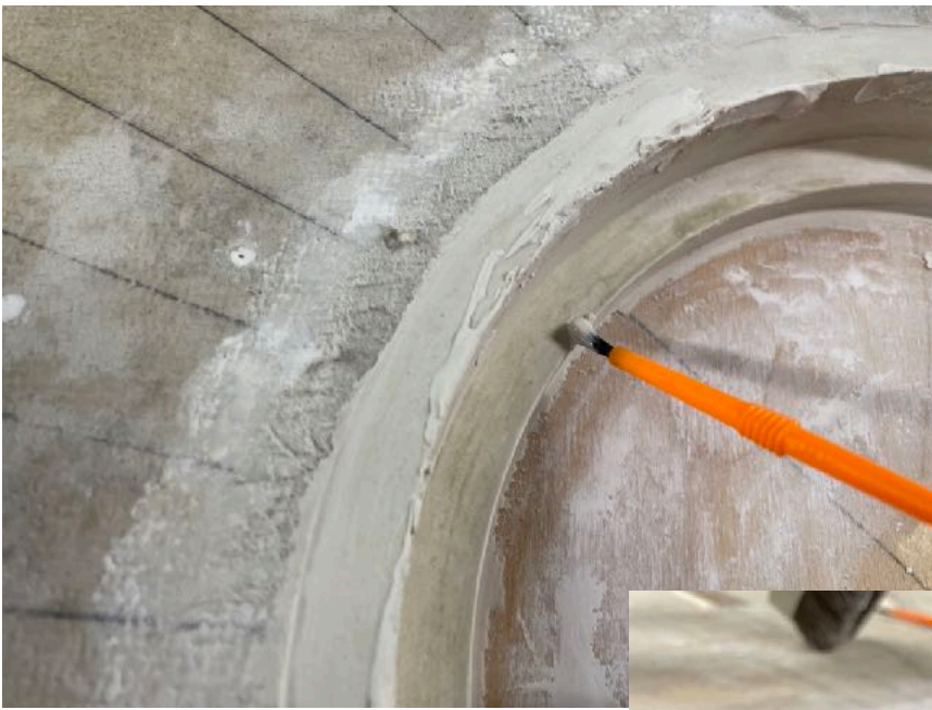
Right: Before and after using my tool to smooth out the final lumps and bumps, a little hand work was required to get an acceptable final contour. I used the forming tool first to check my work and then made a few final passes with it to make things as perfect as I could.
