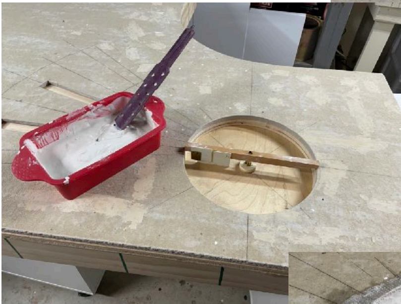
Left: Here is the wet plaster ready to be slopped into place and formed into the first attempt at contouring the pit.
