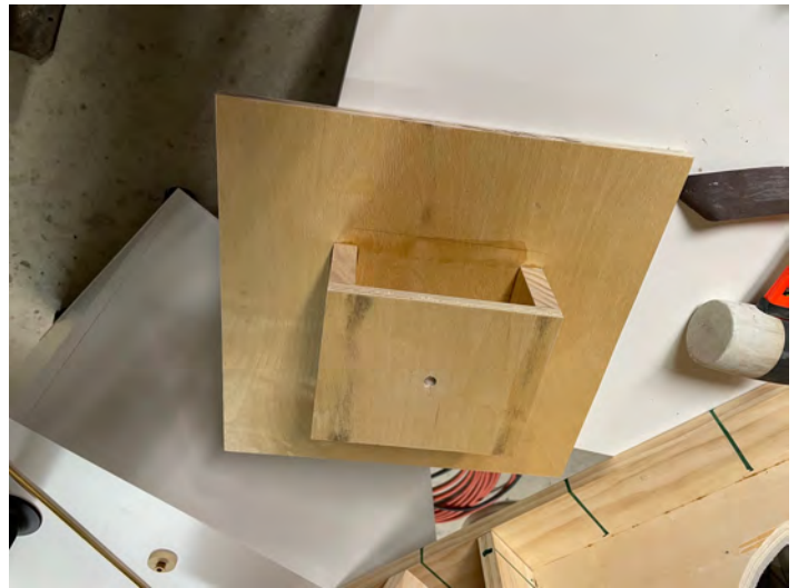
9) I made a lower bearing plate, drilled it, then lined the upper and lower holes as perfectly square as possible.
