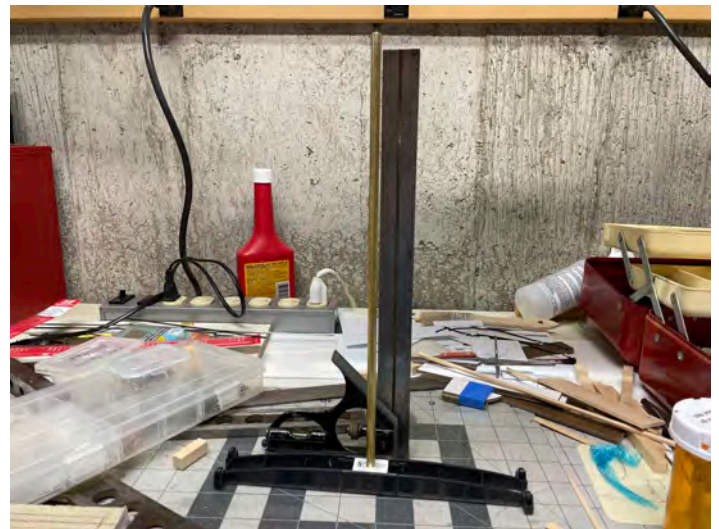
7) I glued the 1/4" brass tube pivot shaft into the turntable bridge making everything as square as possible.
