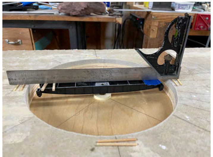
13) After all that, I managed to get the turntable bridge level within two layers of painters tape. Good enough.
