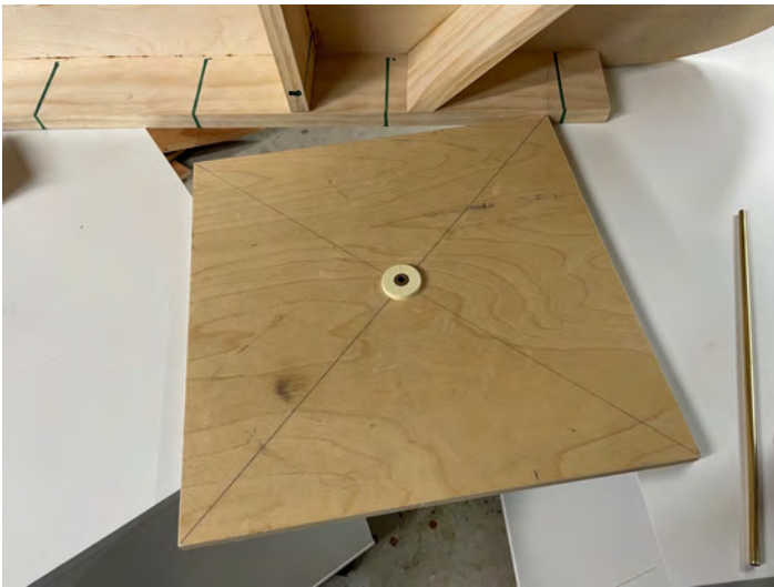
8) Using my drill press, I drilled a bearing hole in the center of a piece of plywood and installed the bearing.
