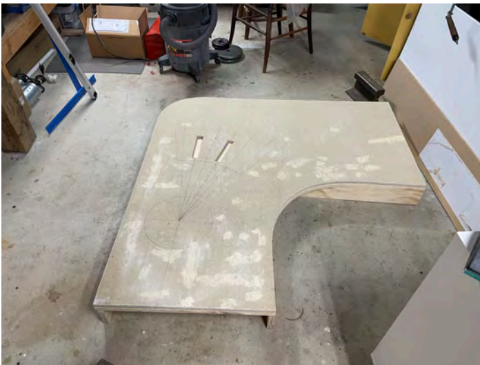
4) When everything seemed to be in the right place, I glued the Homasote to the plywood base.
