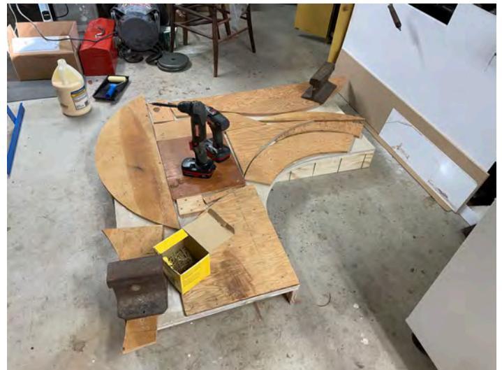
5) Plywood scraps screwed through to the base substituted for clamps while the glue dried.
