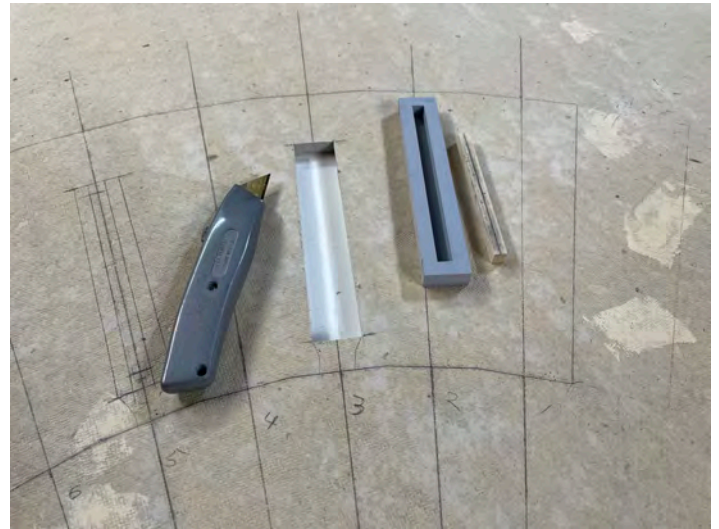
3) I made two inspection pits and cut holes for them before gluing the Homasote to the base.
