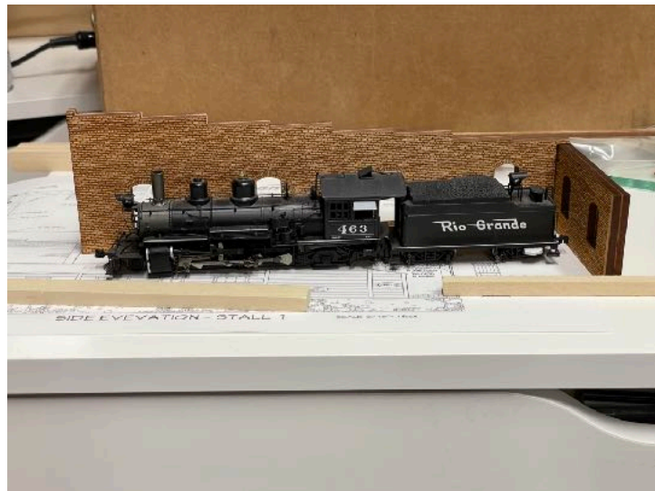
Above: A K-27 locomotive just barely fits lengthwise. A K-28, K-36, or K37 won't. It isn't clearly seen in this picture, but the same is true of height. Below: I cut some back wall pieces to make extensions for longer side walls.
