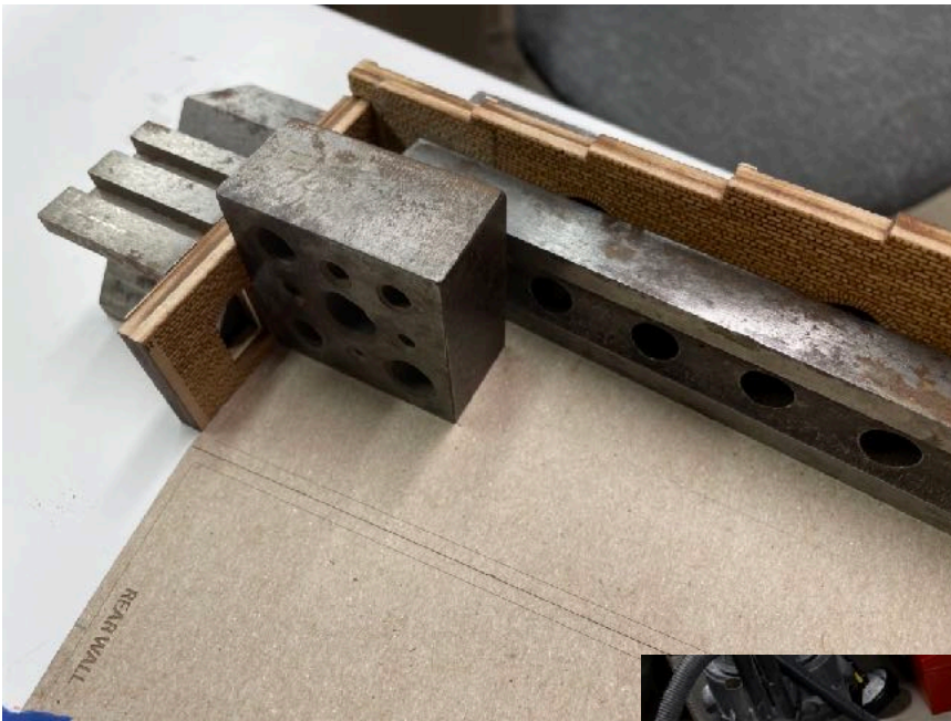
Left: Once I had everything like I wanted it, I glued the back walls to the side walls using the template provided in the kit to get the proper angle.
