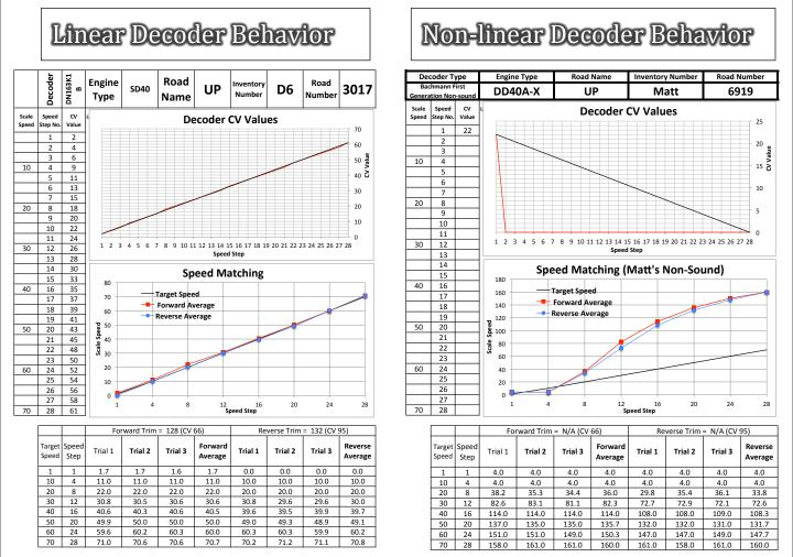
**Caveats:** Sometimes despite all good intentions you "can't get theya from heah" as they say in Maine. Sometimes decoders are very limiting. The second chart (above) shows the results of speed mapping a Bachmann non-sound DD40A-X with factory decoder. There is only one CV that can be programmed – the CV for start speed. "You get what you get" for the remainder of the speed curve. Obviously, if you want to run that locomotive in a consist or DPU'd, the other locomotives would
