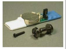
**Computer Products for Education:** This is a device that is mounted in a car and monitors the frequency of the spokes of a wheel as the car moves down the track. A light beam sensor is mounted beneath a car. As the car moves, spokes of a wheel break the light beam. The on-board computer counts how many times the light beam is broken per second and then calculates the speed of the train. http://www.cp4e.com/trsped.htm
