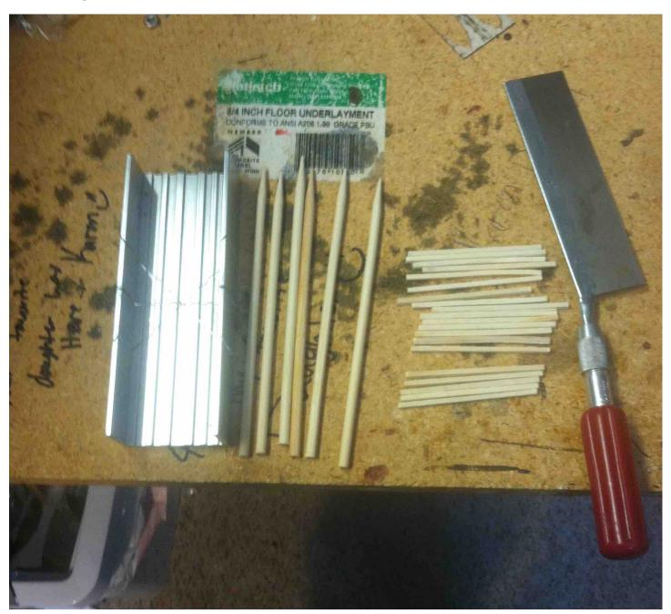
For materials I used wooden food skewers for the bents and craft wood for the ties. The headers on top of the bents and the stringers were made out of oak.
