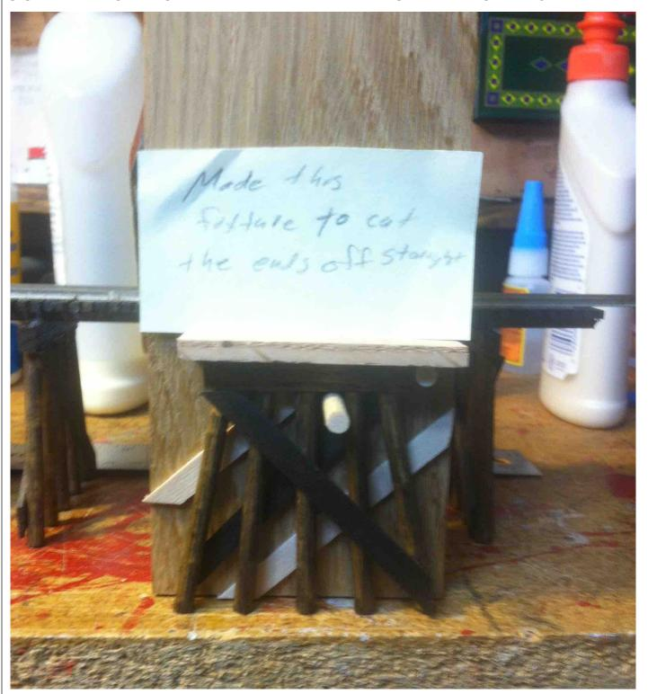
I used Elmer's yellow wood glue. When you are cutting the length of the posts for the bents, use a small miter box and place a block of wood to use as a stop. This will help you keep everything the same length. Also, you will want to use this method for cutting the ties on the deck. Plus you will want to cut the post a little longer than the pattern - about 1/4 of inch. As you look at the pattern, the posts start to make more of an angle on the two outside posts.
