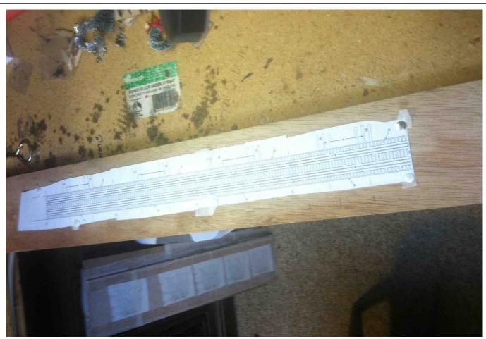
The bridge would be too small for what I wanted or needed. I enlarged and made several copies of the patterns of the bents. First, I cut out the patterns for the bents and glued them on a piece of scrap plywood. Make sure the wood lays flat on the bents and the deck. Next, I taped down wax
