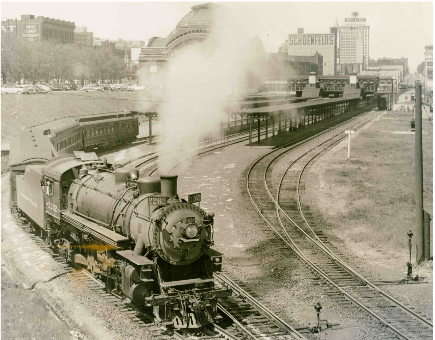
This is a view of Northern Pacific 2262, a 4-6-2 Q-6 on May 18, 1954. The locomotive was built in 1923. It is shown on train 415 departing Tacoma Station on train #415. Up until August 25, 1954 this "stub" faithfully handled Tacoma passengers and baggage to and from East Auburn. This train was replaced by a bus.
