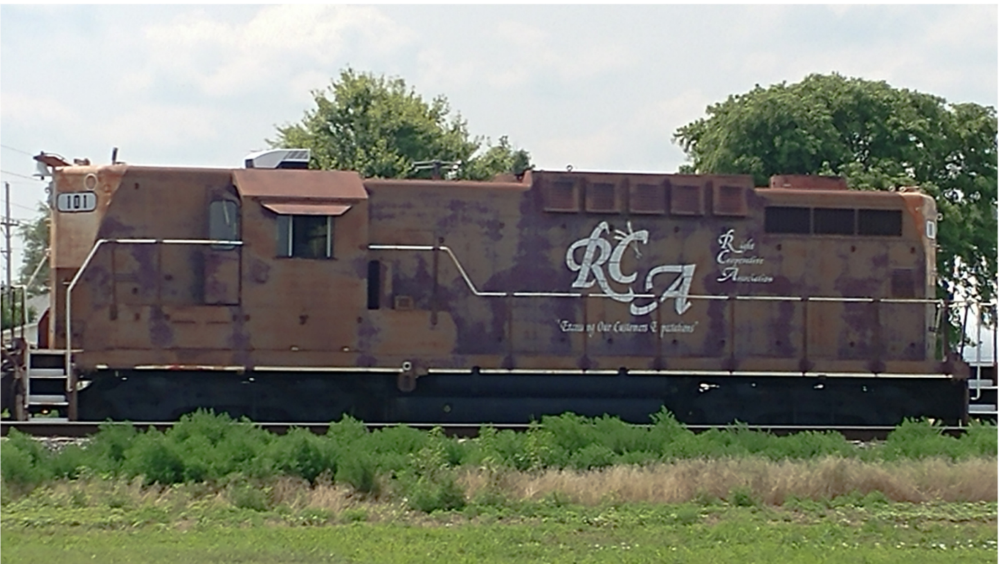
(Above) The RCAX 101 began life in November 1958 as Norfolk & Western 519, a EMD GP9. After the merger into Norfolk Southern the 519 was rebuilt into an EMD TC-10 featuring a 1050 HP Caterpillar prime mover. Now wearing the colors of the Right Co-Op Association, it is paired with the 1702 and is operated by remote control from the elevator loading platform.
