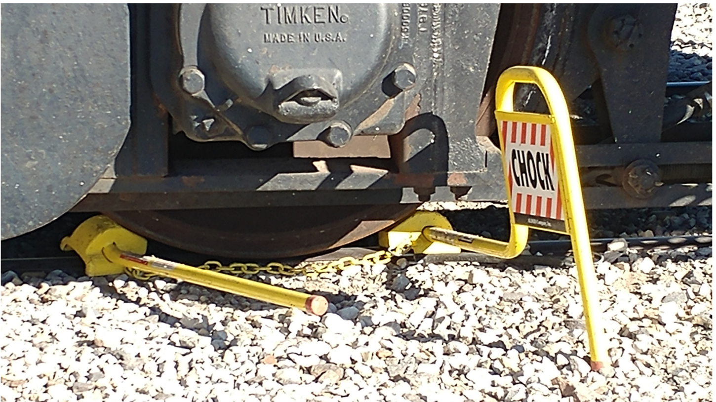
(Below) The wheel chock used on the front truck.
