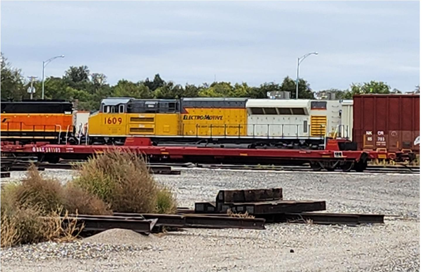
10/7/22 I came across this Electromotive in the BNSF Dodge City yard today. It's an Electro Motive SD70ACe-T4 rebuilt from a SD70ACe to Tier 4 standards. The 1609 is one of the first demos out of production. Looks like it underwent cooling modifications for testing out at Pueblo as it is part of a westbound consist.
