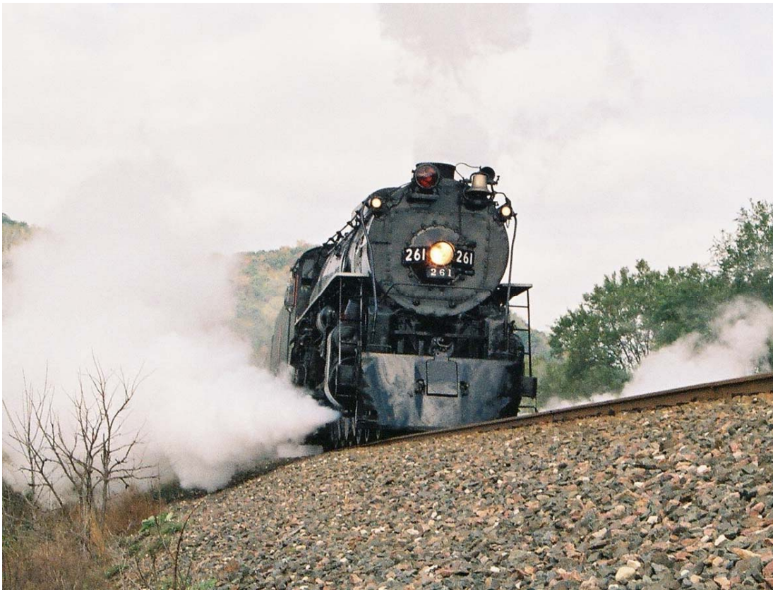
261 going through a cylinder blow down.
