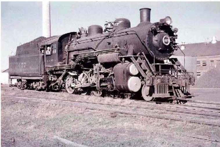
*This engineer's side view shows the running gear and piping very well. Note the footboards on the front pilot.*
