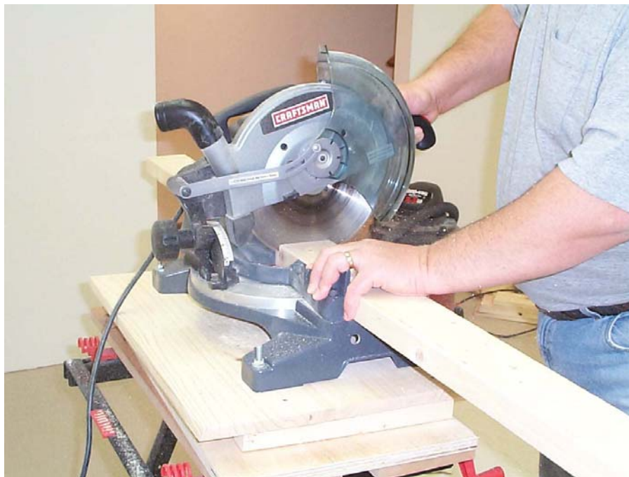
Here I am cutting 28-inch lengths of 2 x 4s that will be screwed to the bottom of the literature organizer.
