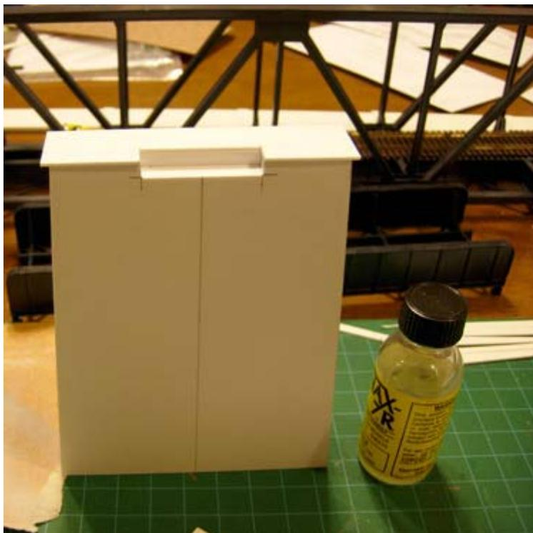
**Test fitting the pier cap prior to final assembly.**
