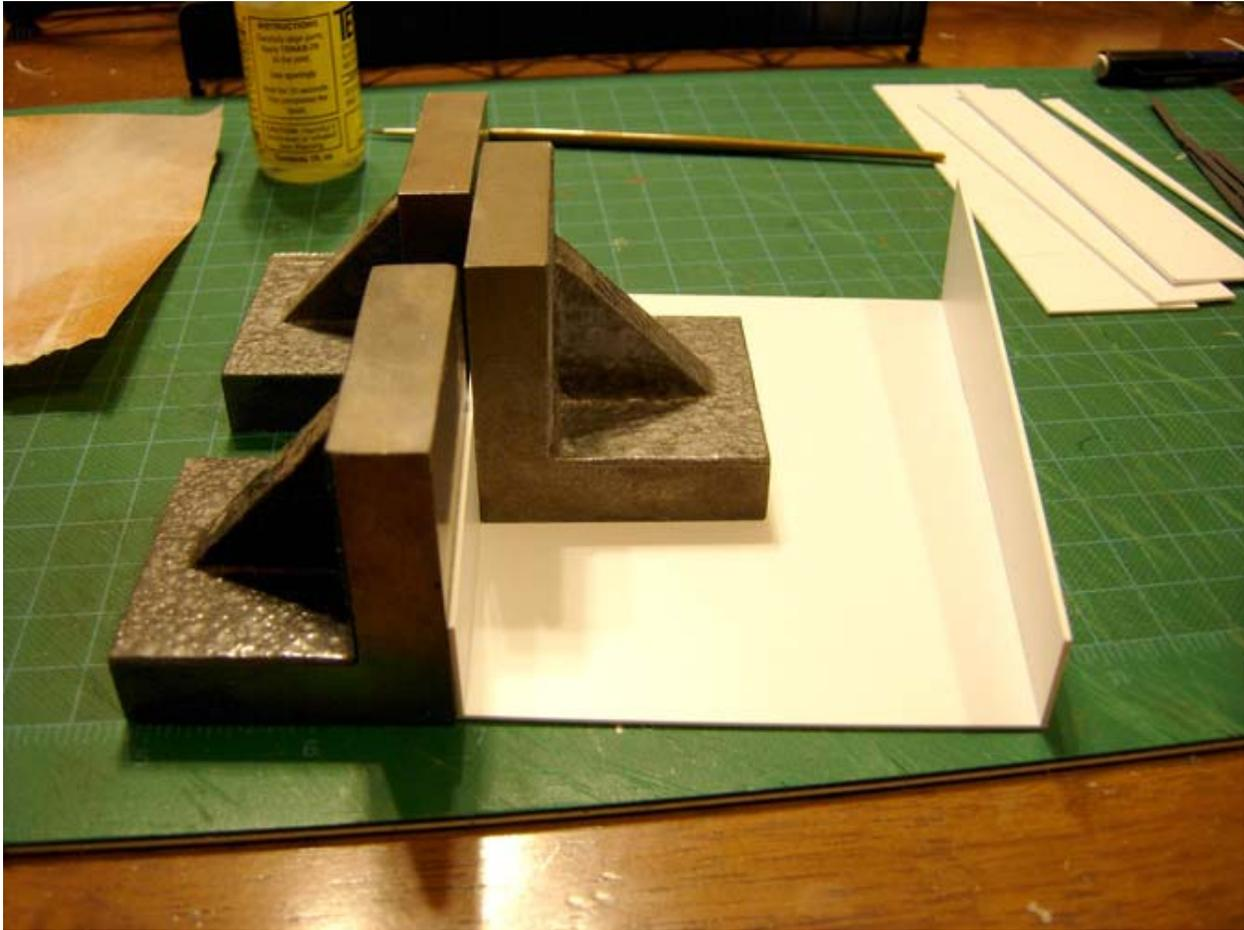
To assemble the pieces, I used 2x2x2 steel Angle Plates, available from Micro-Mark, to hold them in place. The configuration of the three plates will produce perfect 90-degree angles with very little joint clean up.
