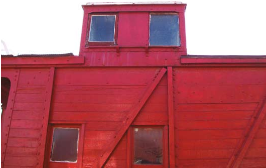
Here are two views of the cupola from a passenger / baggage caboose located in Walker, Iowa. The roof walks around the cupola and down the center of the roof are missing, but you can see the all steel construction of the cupola that were the same on the standard and passenger / baggage cabooses. Unfortunately this caboose has had its roof replaced with sheet metal instead of the wood roof with tarpaper.
