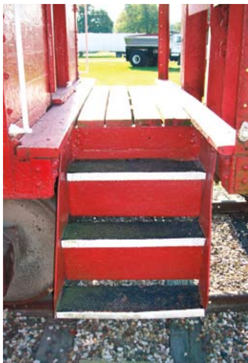
A view of the passenger / baggage end of the caboose shows that the truck has been inset from the end of the car on the center sill to accommodate the passenger style steps.
