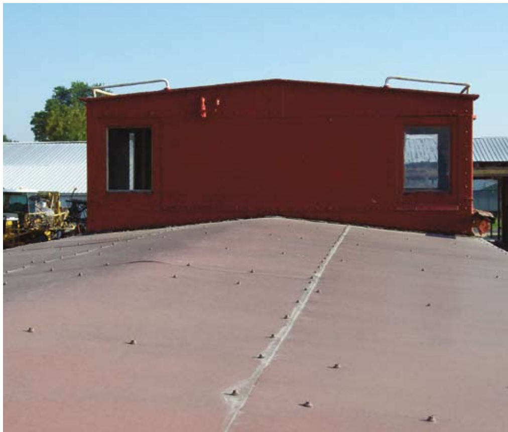
Here are two views of the cupola from a passenger / baggage caboose located in Walker, Iowa. The roof walks around the cupola and down the center of the roof are missing, but you can see the all steel construction of the cupola that were the same on the standard and passenger / baggage cabooses. Unfortunately this caboose has had its roof replaced with sheet metal instead of the wood roof with tarpaper.
