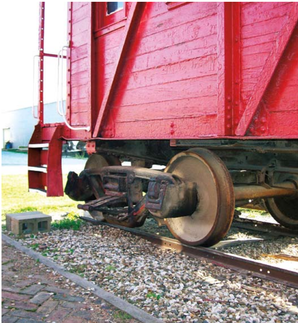
On the freight end the truck was not moved and the steps were more of a ladder style step mounted on the outside frame of the caboose. You can also see the "Z" angle bracing of the caboose. I had to change my plans for this bracing when it looked too bulky for an N scale model.
