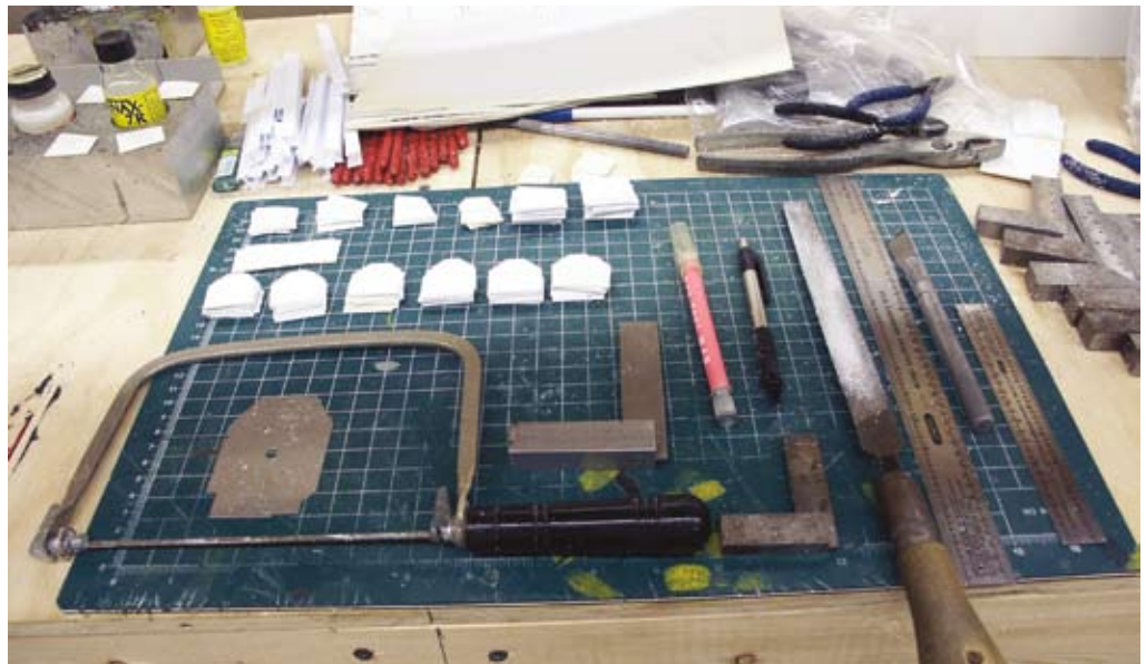
Above: Richard used simple hand tools to build this bridge: a scale ruler, a flat bastard file, an X-acto knife with No. 11 blade, a pencil, machinist squares, a coping saw, a miter box, and a modified copper one. The various styrene shapes in the upper left corner of the green pad are many of the custom-cut splice plates for the bridge.
