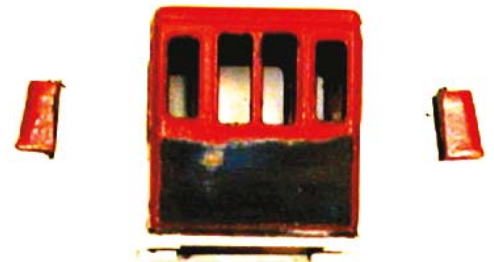
Above: The Bachmann GE-44 tonner cab was modified by lowering it and removing the stock exhausts. The cab sits on a 0.030-inch sheet of styrene.
