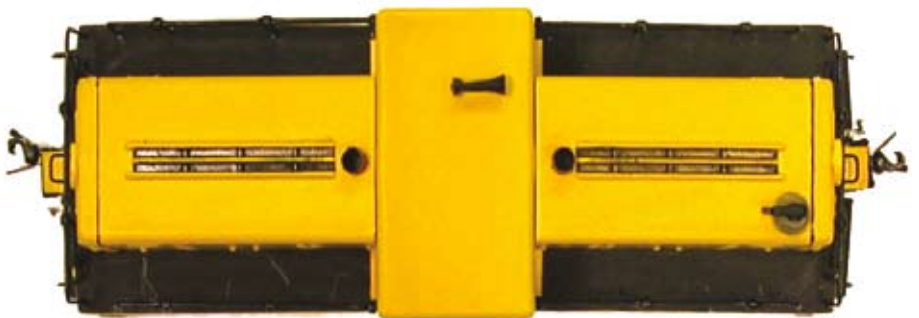
ABOVE: This down-on shot clearly shows the detail additions added during the modification of the locomotive. The exhaust pipes, smaller couplers, and the hood-mounted bell add to the visual character of the little switcher.
