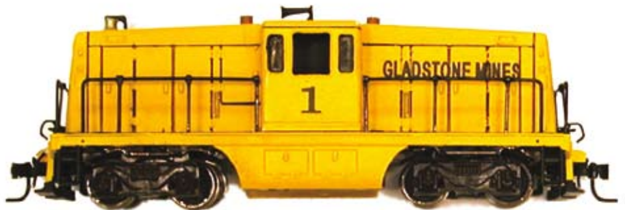
ABOVE: The N scale GP40 underframe and mechanism were super-modified to fit inside of a kitbashed GE 44 tonner shell. Number 1 brings a little diesel action to the HOn3 steam on the layout. The wheelbase of the new unit is 2.520 inches, a little shorter than that of the 44-tonner.
