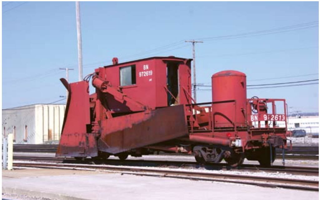
All Above: BN 972619 sat at Murray Yard in Kansas City in 2004. This is a "Standard model 2-200" and had been well-maintained by the railroad. Its upgrades include roller-bearing trucks and a modernized cab. Notice the rear-mounted air reservoir and the center-mounted cab. A sharp eye will pick out the extra air hose on the rear of the spreader used to tie into the locomotive air system to charge the pneumatic tank on the spreader. That means this spreader depends on the motive power to operate. Stephen M. Priest, photos
