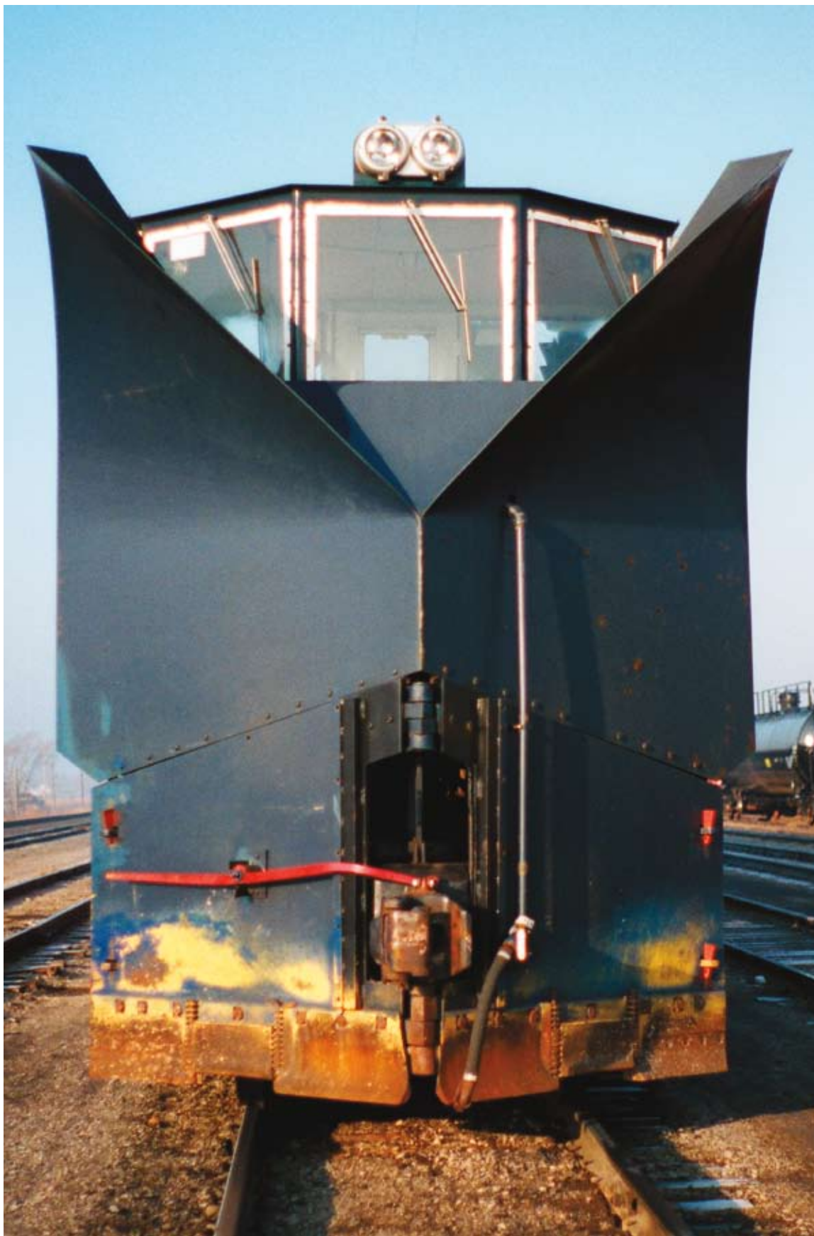
Right: AT (ATSF) 199255 sat at Emporia, Kansas. The high snow blade is impressive from this angle. The red lever is used to pull the pin on the coupler. Stephen M. Priest, photo
