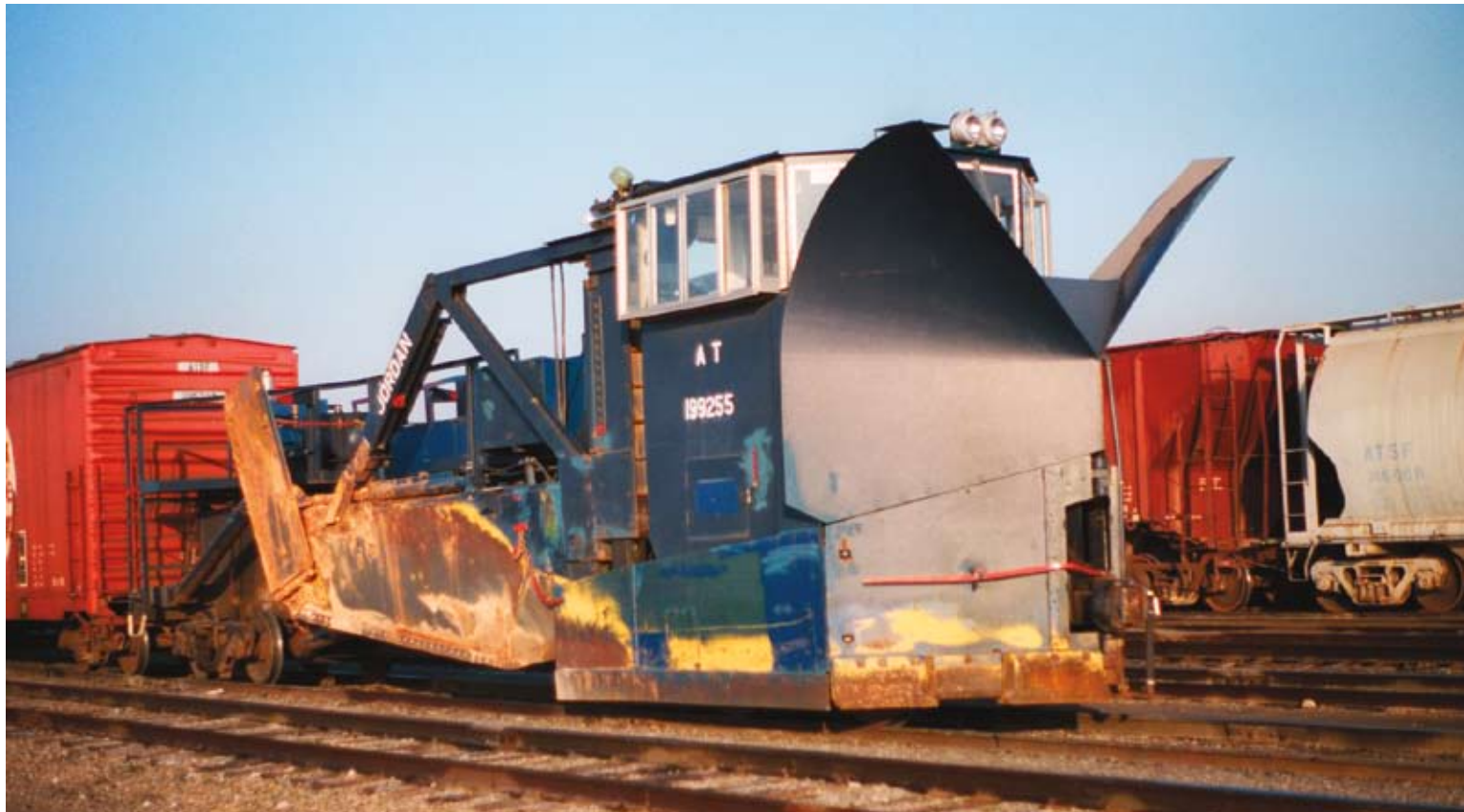
ABOVE: AT (ATSF) 199255 is a Type-J with a raised rear deck and complete self-contained hydraulic system. The front cab and high "snow blade" options are also visible. Stephen M. Priest, photo
