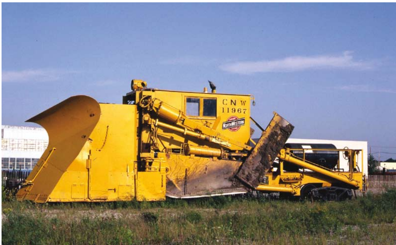
Below: CNW 11967 appears to have been recently rebuilt and painted. This is also a "Standard 2-200" model with a horizontal air reservoir and a split sloping wing. Notice the journal access doors on the side of the front plow. Tom Farrell photograph
