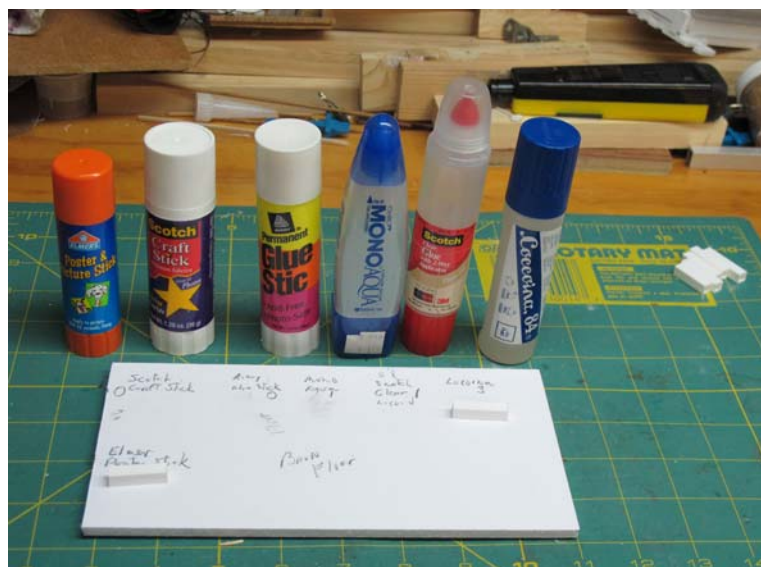
Figure 1 Test of non-repositional glue sticks. Only two of the six bonds survived a light nudge. This piece of Gatorfoam board had already been cut to serve as the floor of the barn.
