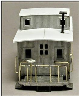
using a bending jig from an old AMB kit. The windows are made from Micro Scale Micro Crystal Klear. I installed mechanical brakes because this kit was so short there was no room for a type K brake cylinder. Since this was a short line home built caboose for the old Webster Groves & Fenton, I used a set of friction bearing freight trucks. A set of Kadee whisker spring couplers completed the job. I made the banner
