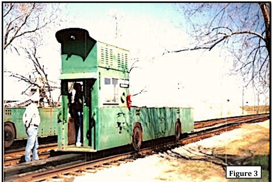
Figure 3 A small cab in the front where the operators would stand. The louvered area above the cab is, I believe, where all the relays and capacitors for the controls would be. The little round silver disc behind the cab window is a spot light. This view shows the bi-fold door used to allow access to the operators cab and the cover over the electrified rail in-between the rails is visible too.
