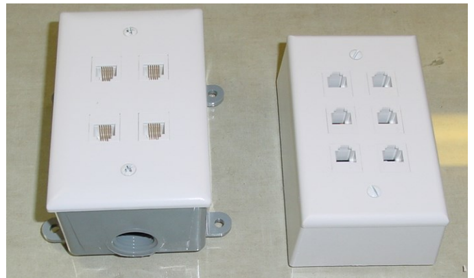
Figure 5 Completed Loconet Hub boxes
