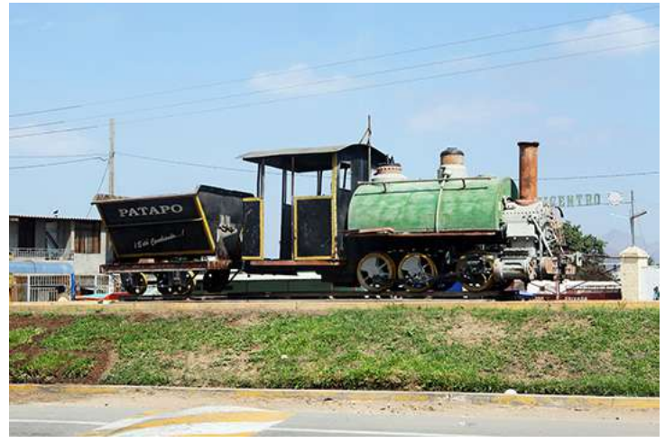
A 700 mm narrow gauge sugar cane locomotive and car on display in the town of Pátapo in northern Peru.
