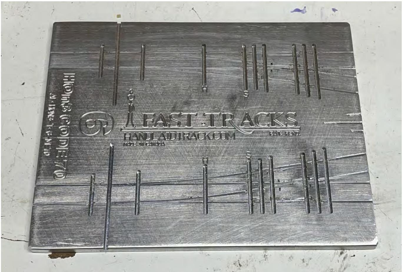
This Fast Tracks assembly fixture is the one I use. It is a #6 HOn3 for making left and right hand switches. I suspect you can imagine how quickly it can take the heat out of the rail you are trying to solder. Practice has helped, but it's still a little tricky for me.
