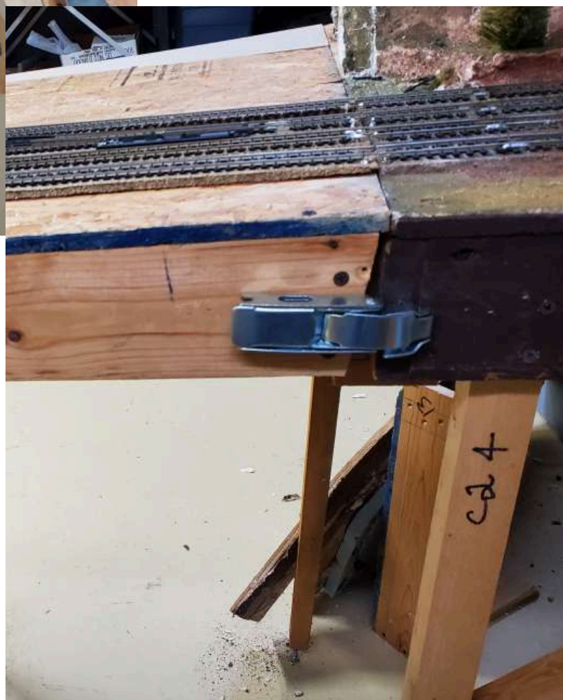
A draw latch on the unhinged end worked well for holding the lift-up section tight against the rest of the layout. However, it couldn't be reached once you were inside the layout. This will be moved to the top side to be accessible from both inside and outside of the layout. I will have to figure out how to hide it.
