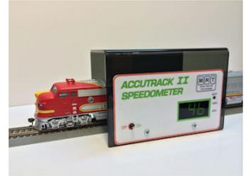
**Arduino Microcomputer Speed Trap:** This is a speed trap built on an Arduino microcomputer that calculates train speed based on distance between sensors and time to traverse the distance.
