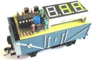
**Home made Hall effect sensor:** Custom made for a particular installation and measures wheel rotation over time to yield train speed. Requires assembly, as only the description of the device is given here:
