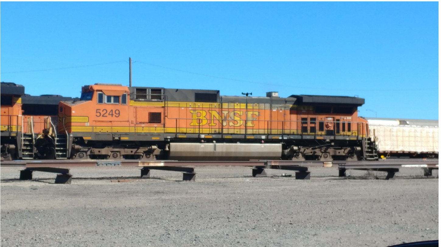
(Below) BNSF 5249 is a GE is a C44-9W that was new in 2002.
