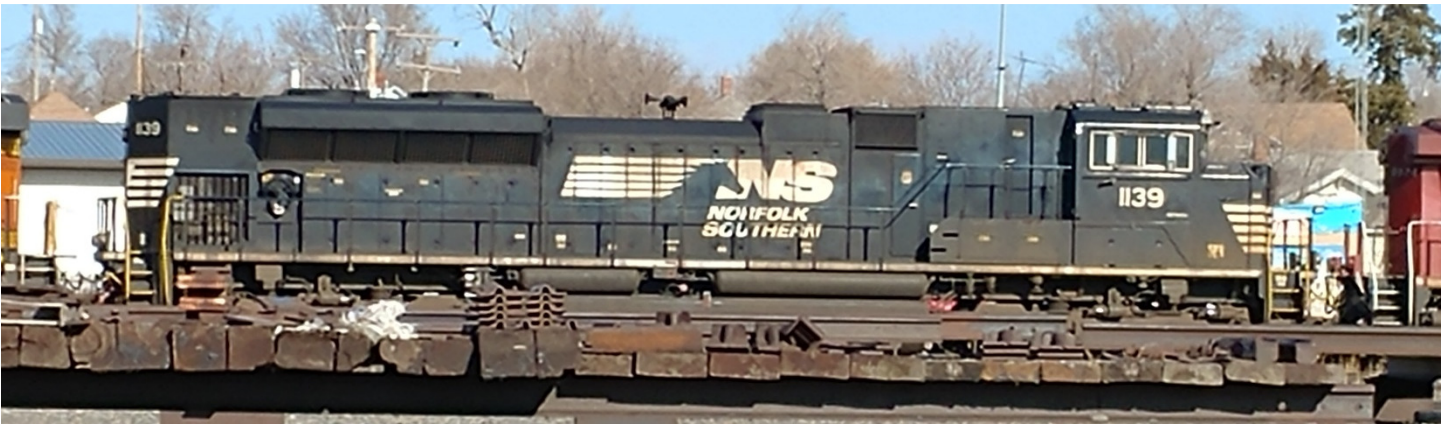
Norfolk Southern 1139 was constructed in November of 2014 by EMD as a SD70ACe .
