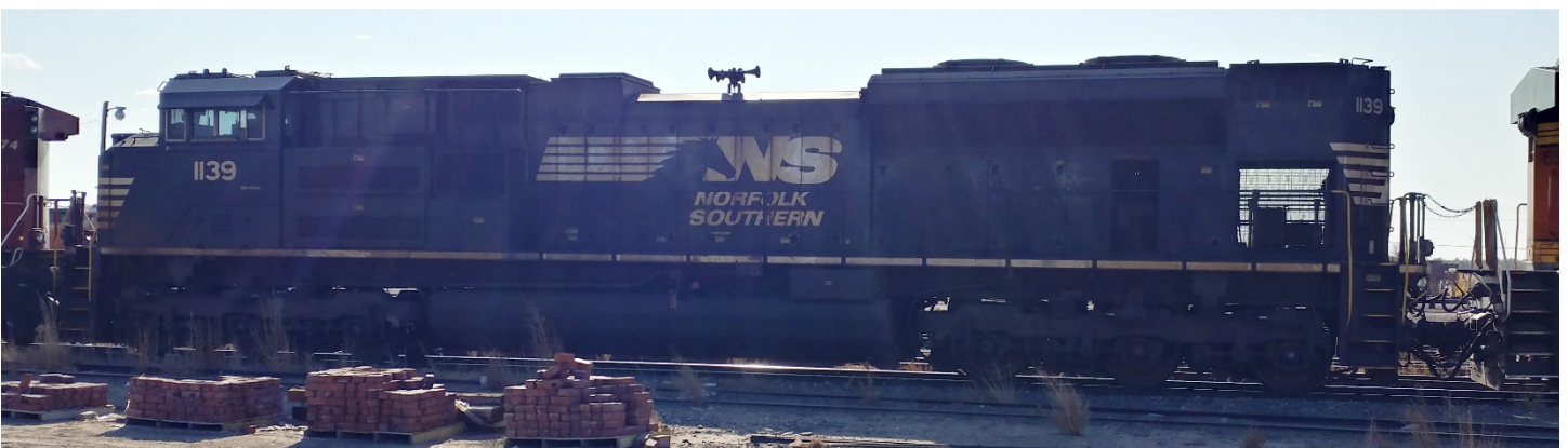
Norfolk Southern 1139 was constructed in November of 2014 by EMD as a SD70ACe .
