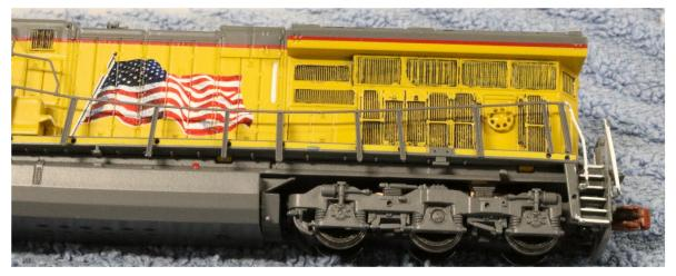
(Above) Once you have "erased" and "de-crumbed" all the grills, it's time to reinstall the handrails. You can see the holes where the pins go, so we like to start in the middle and work out to each end. Use tweezers to align the pins with the holes and gently push back in.
