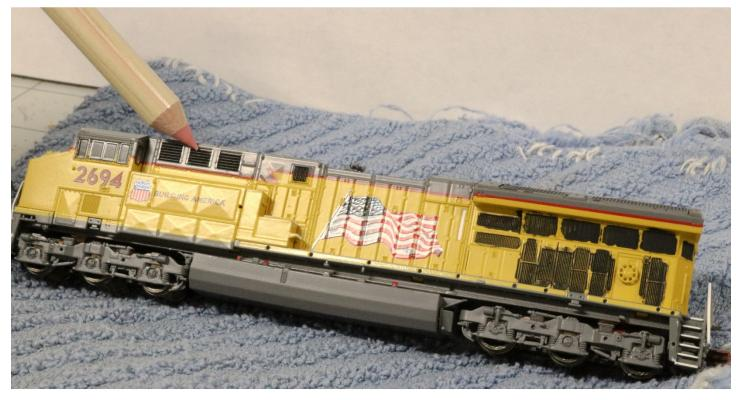
(Above) This is one reason we prefer eraser pencils as you can see the fine point which will get into small crevices. We started with the dynamic brake grills behind the cab. Hold the loco firmly with one hand and begin to rub on the grills starting with light pressure until you gain some confidence. You need to make sure your eraser is a smooth type with no grit added as a "Bright Boy" or gritty eraser may rub through the original paint as well.
