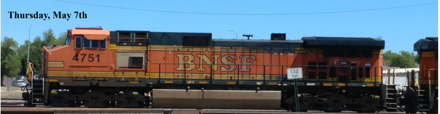
(Above) BNSF 4751 was built in March of 1998 as a GE C44-9W.
