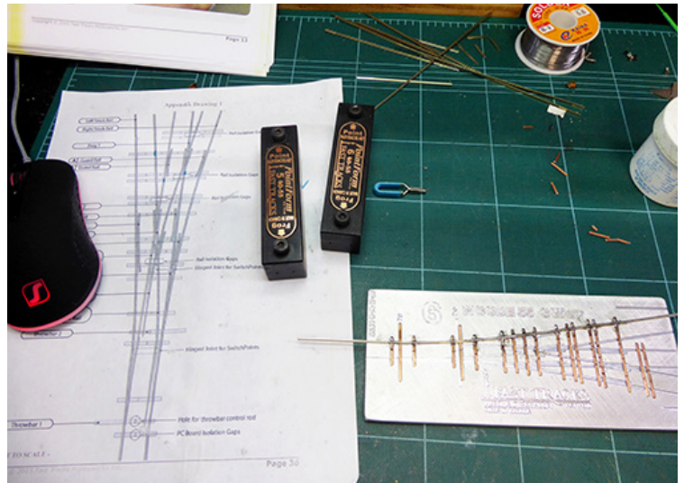
Figure 3 Civil Engineer: Using a layout jig to build a three way turnout
