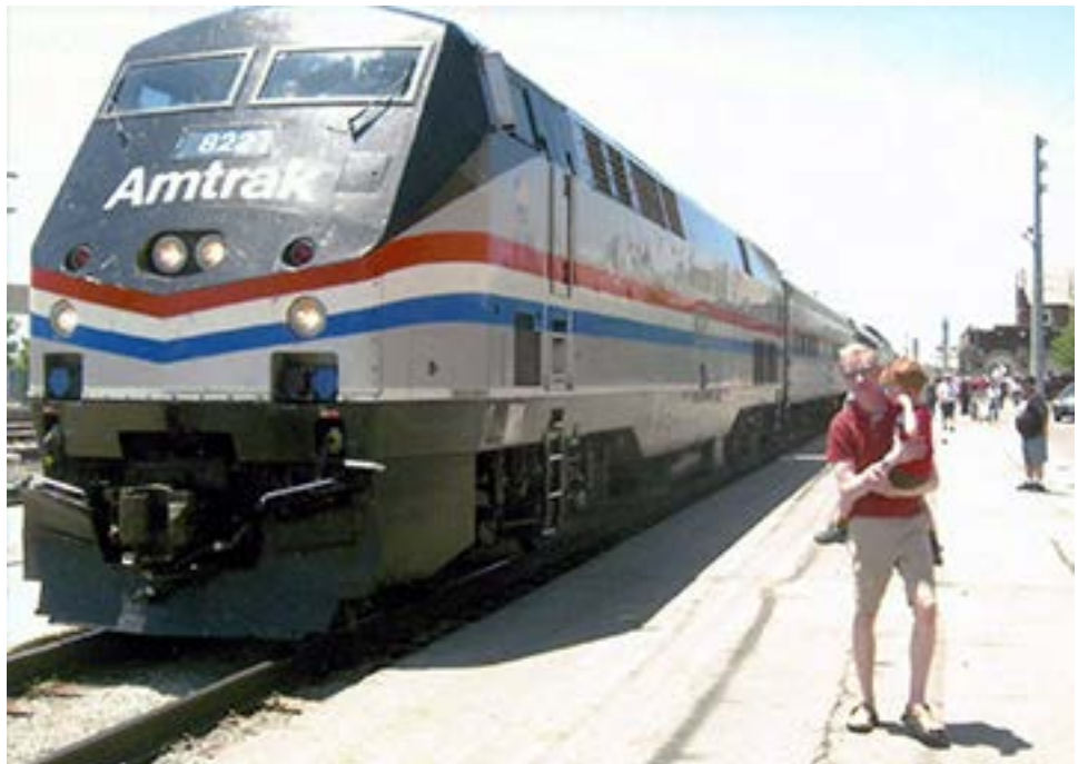
Front of Inspection train - entire consist: Amtrak P40 #822; Amtrak passenger car (Crew Quarters); Viewliner passenger car; Full-length dome car (the "Ocean View"); and Viewliner inspection car.
