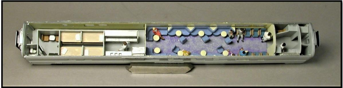
the kitchen, bunk room crew lounge/locker room, and restroom. The kitchen/dormitory end is designed to hold a crew of 10. On overnight trains, the bunks could accommodate 8. Two of the crew on duty to service the passengers during the night.
