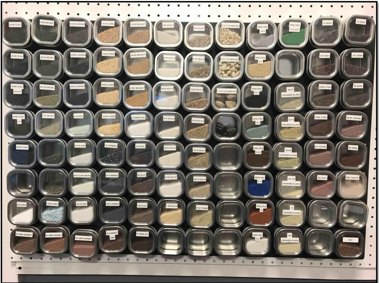
Some of the media were artificially colored (third and fourth column from the right), but most were the natural colors that nature had given the media. (Note, the colored samples are used in mortar to yield the desired uniform color specified by the architect. And it is very uniform in color.)
