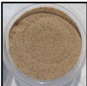
**Mason's Sand Quickrete brand:** Approximately \$7.00 per 80-pound bag. It conforms to ASTM C-144, which means that the particle size is screened to a sieve (or mesh) size of approximately 30 to 50. More on sieve (mesh) size later. I have found that this color is not correct for any of the prototype RR's I am modeling.
